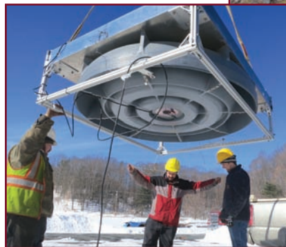
Creare personnel prepare to test the prototype CAAT suspended from a construction crane.
