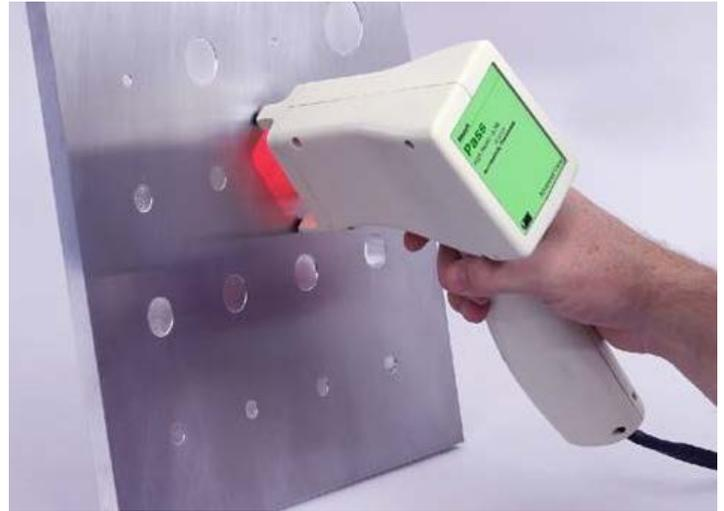
Handheld measuring head and calibration plate
