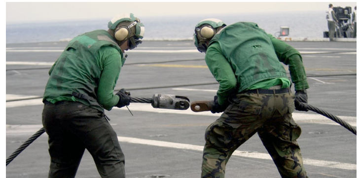
Flight deck sailors attach a new arresting cable to the arresting gear assembly (US Navy photo by Andre Rhoden / Released)
