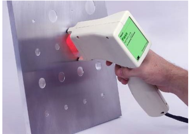
Handheld measuring head and calibration plate
