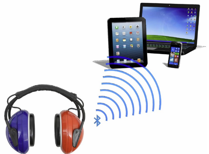
The Creare headset connects wirelessly to software on a smartphone, tablet, or laptop
