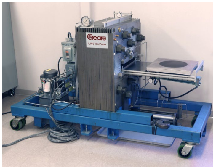
1700-ton stamping press for producing heat exchanger plates
