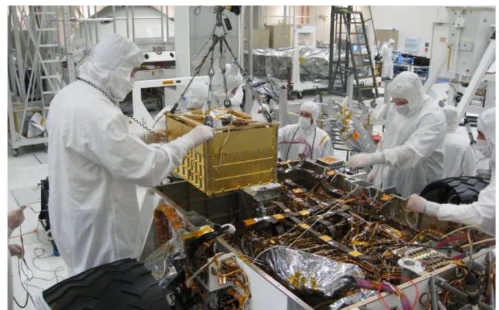
Installing the Sample Analysis at Mars instrument package in the Curiosity rover
