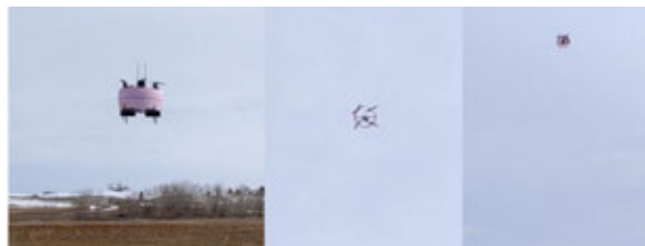
Figure 2. Titan Ringlet Drone in Hover (left), Transition Flight (center), and Cruise Flight (right).
