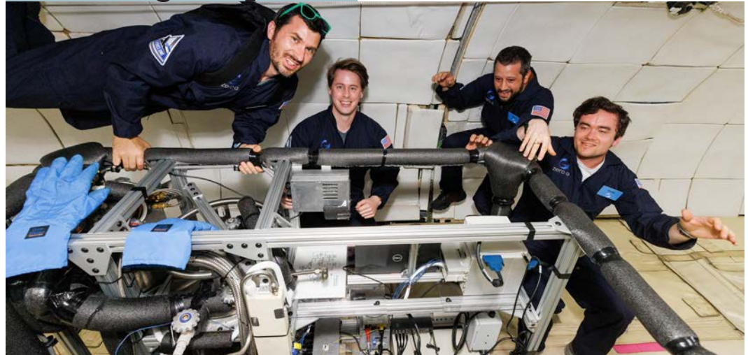
Testing the Hybrid LAD in Microgravity (Photo courtesy of Steve Boxall, Zero-G)
